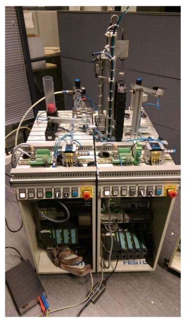
Figure 1 Distribution station (left) and testing station (right)
