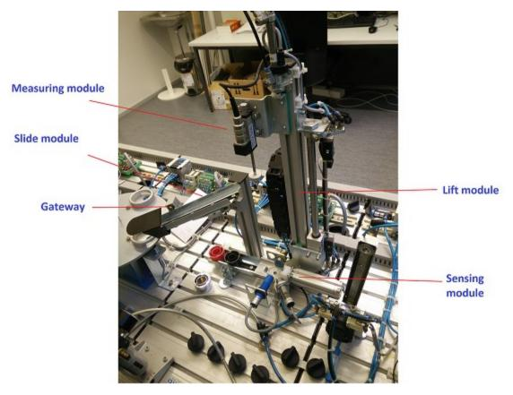
Figure 10 Modules of Testing Station.
