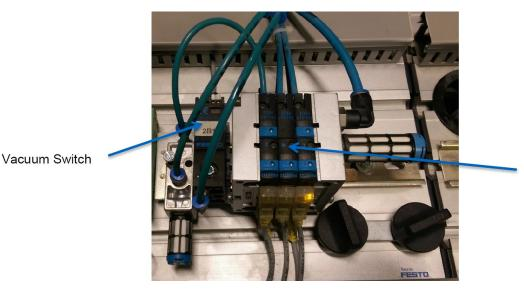
From left to right, 5/2-way valve, Vacuum Generator, 3/2 way valve
