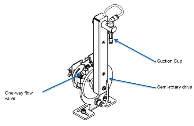
Figure 6 Rotary drive module
