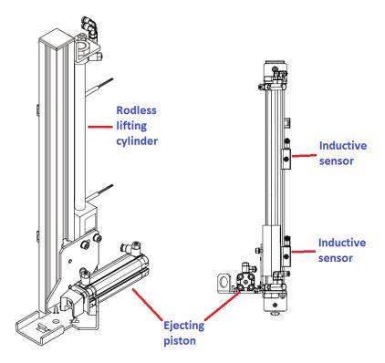
Figure 12 Lift module
