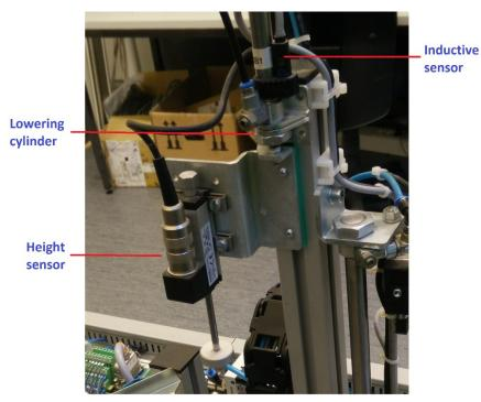
Figure 13 Measuring module
