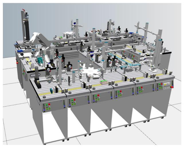
Figure 2 MPS workstation forming a complex production line. The distribution and testing stations in Figure 1 are on the left in the foreground
