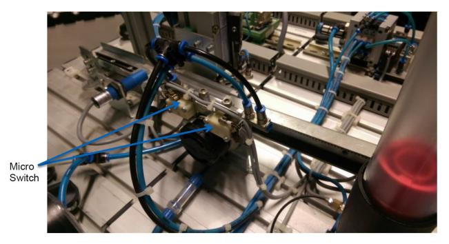
Figure 7 Back side of rotary drive module, showing the micro-switches
