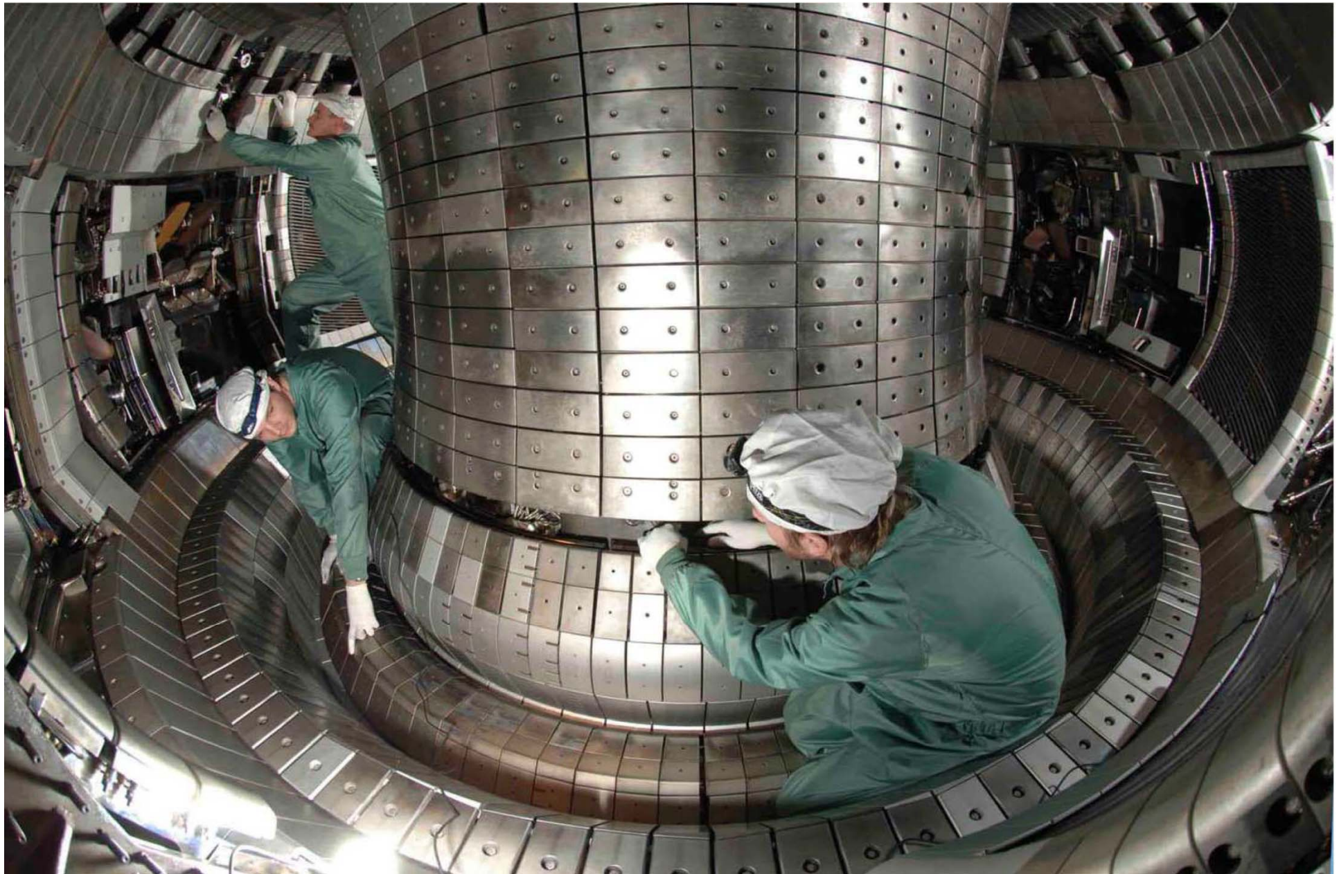
Interior of ASDEX Upgrade – Since 2007 full-W wall
