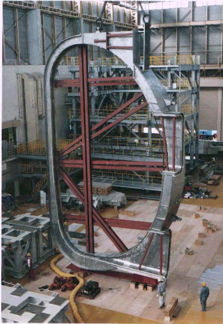
section of the vacuum vessel (1/20)
