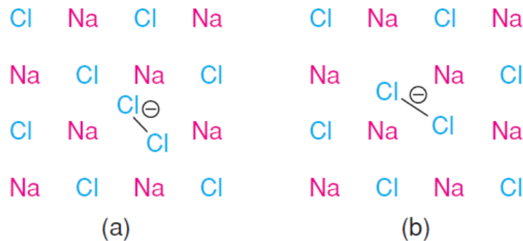
Figure 2.6 (a) H-centre and (b) V-centre in NaCl.
