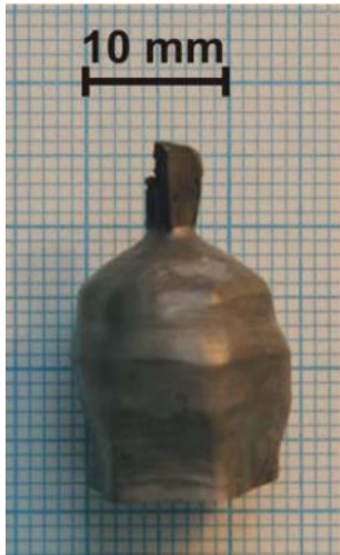
13 gram single crystal of \text{Ba}_8[\text{Ga}_{16}\text{Ge}_{30}]
