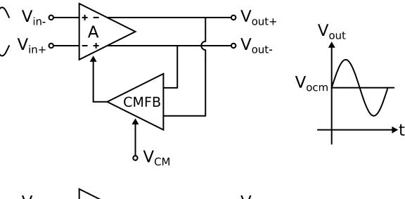
Common-mode feedback does not affect the differential signal.
