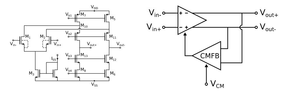
CMFB:common-mode feedback amplifier (error amplifier)V\_{CM}:external common-mode voltage
