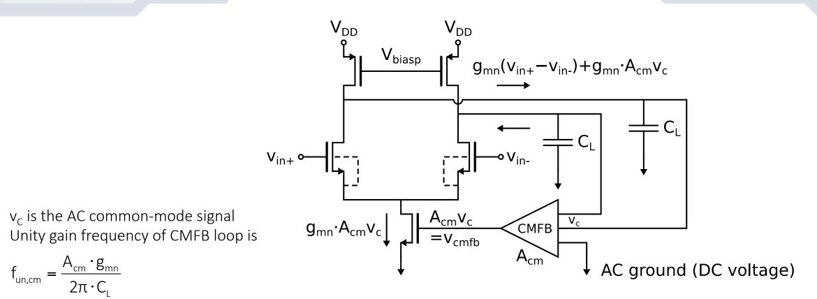
If we want to compensate the CMFB loop with the same load capacitance used to compensate ٠ the differential forward signal path, then we must ensure that the gain of the CMFB amplifier is
