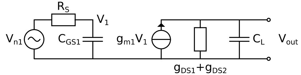
$$A_{n1} = \frac{V_{on1}}{V_{n1}} = \frac{-g_m}{(sC_{GS1}R_s + 1)(sC_L + g_{DS1} + g_{DS2})}$$
