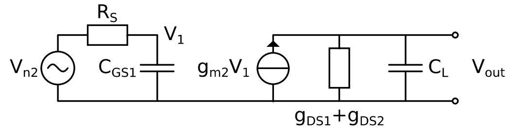
$$A_{n2} = \frac{V_{on2}}{V_{n2}} = \frac{-g_m}{(sC_{GS2}R_B + 1)(sC_L + g_{DS1} + g_{DS2})}$$
