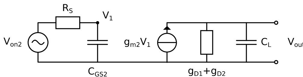
$$A(s) = \frac{-g_{m2}}{(sC_{GS}R_s + 1)(sC_L + g_{D1} + g_{D2})}$$
