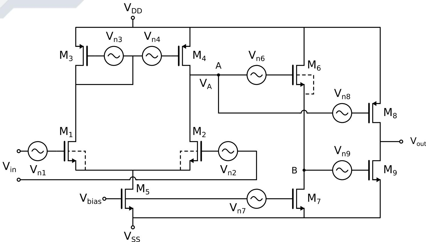
Noise reduced to the inputs of different stages
