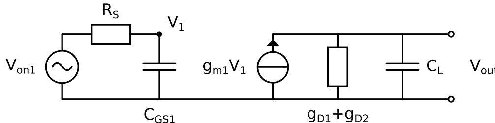
$$A(s) = \frac{-g_{m1}}{(sC_{GS}R_s + 1)(sC_L + g_{D1} + g_{D2})}$$
