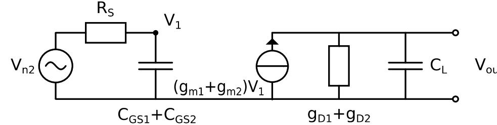
$$A(s) = \frac{-(g_{m1} + g_{m2})}{(s(C_{GS1} + C_{GS2})R_s + 1)(sC_L + g_{D1} + g_{D2})}$$
