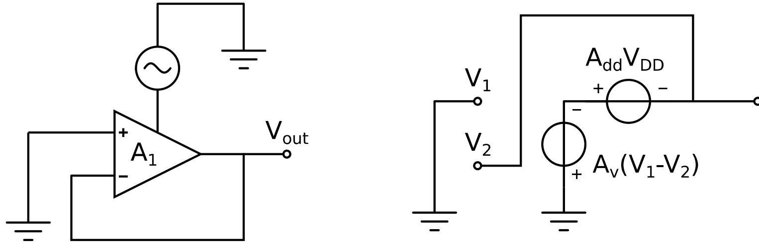
$$V_{out} = \frac{A_{dd}}{1 + A_v} V_{dd} \approx \frac{A_{dd}}{A_v} V_{dd} = \frac{1}{PSRR} V_{dd}$$
