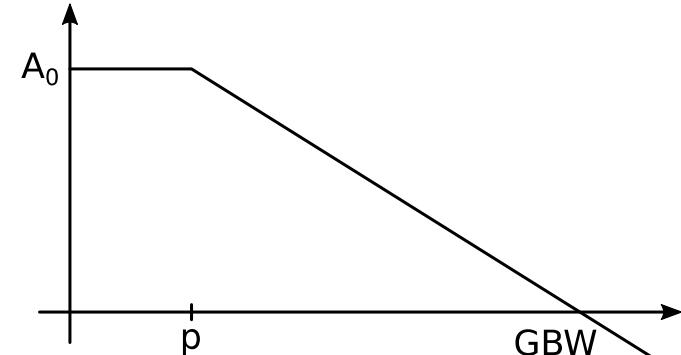
$$\frac{V_{out}}{v_{ns}} = \frac{1}{1 + \frac{s}{GBW}}$$
