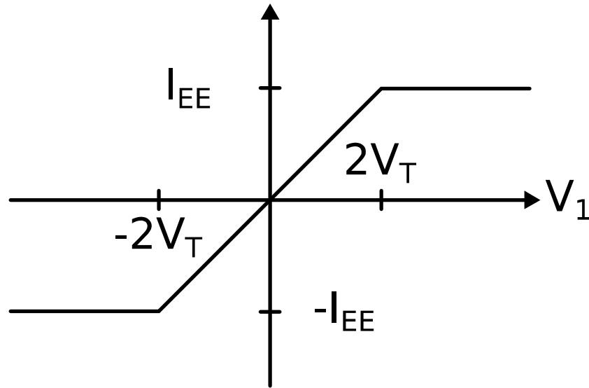
$$I_{C3} = \frac{I_{EE}}{\left[1 + \exp\left(\frac{-V_1}{V_T}\right)\right] \left[1 + \exp\left(\frac{-V_2}{V_T}\right)\right]}$$
