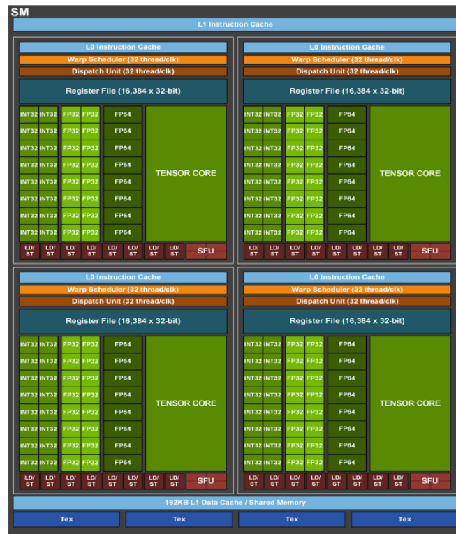
Figure 2. GA100 Streaming Multiprocessor (SM) [8]
