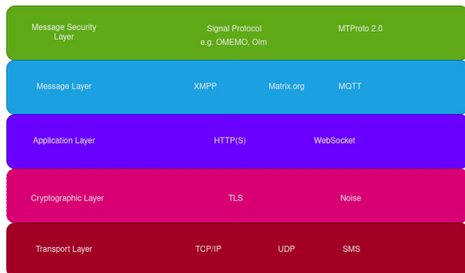
Figure 1. The instant messaging protocol stack.
