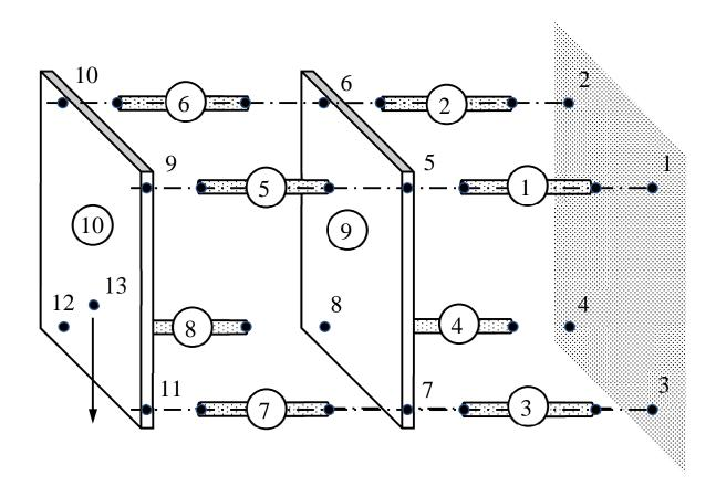
The book-keeping with unique identifiers for the structural parts and connection points allow a consistent naming of the kinematic and kinetic quantities of analysis.
