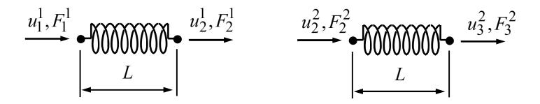
• Interaction model between the bars and with the surroundings is of type "fixed" so  $u_1^1 = 0$ ,  $u_2^1 = u_2^2$ , and  $u_3^2 = a$  (left edge welding, integrity of structure at the connection, and displacement of the right end wall). The force constraints are due to Newton III
