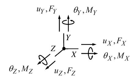
Vector quantities are invariants in the sense  $\vec{a} = a_x \vec{i} + a_y \vec{j} + a_z \vec{k} = a_X \vec{I} + a_Y \vec{J} + a_Z \vec{K}$ , and can be transformed from one coordinate system to another using the property.
