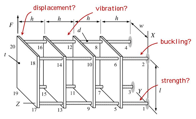
Displacement and stress analysis according to the linear elasticity theory may not entirely explain the behavior of a structure!
