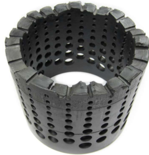
Fractured steam diffuser, material X35CrMo17 martensitic stainless steel
