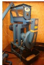
SPC pelletizer, mounted in a container system.
