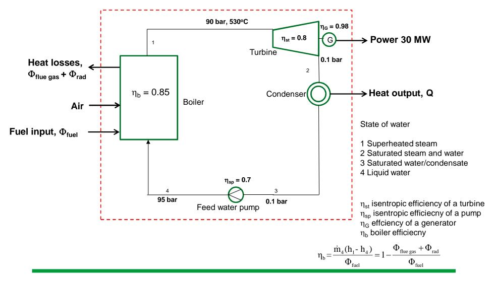
$\Phi_{fuel} = \dot{m}_{fuel} LHV$ LHV = lower heating value of fuel
