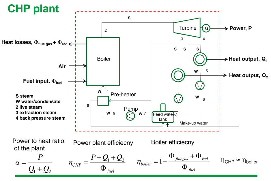
Aalto-yliopisto Insinööritieteiden korkeakoulu Auxiliary systems of the power plant (e.g. flue gas fans, air fans, fuel processing systems) consume electricity which must be taken into account in accurate calculations.
