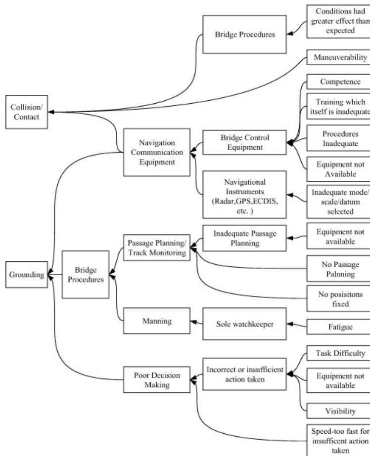
Example: Fault tree diagram from a marine accident
