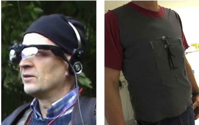
Fig. 1. Wearable devices. Left: HMD for presenting visual modality. The light-weight headphones were used in Study 1 and in the bimodal VA condition in Study 2. Right: Tactile vest showing three rings of factors.
