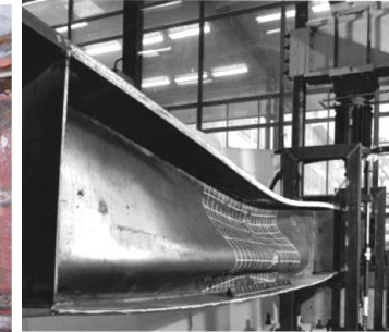
Figure 2. Vertical web buckling.
