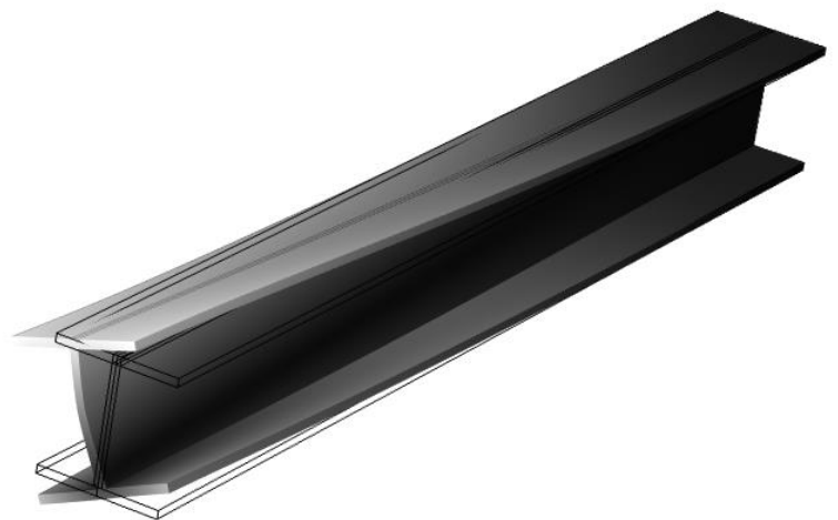
Lateral buckling of I-beam cantilever
