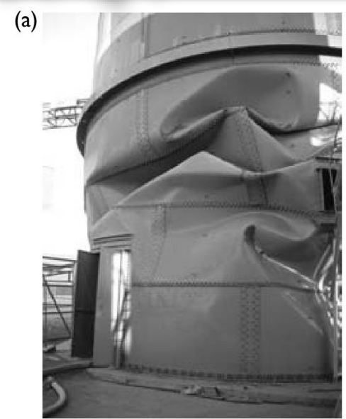
Figure 2.4 Typical appearance of axial compression buckles: (a) failure in service; (b) test in laboratory (Knödel and Schulz 1992).
