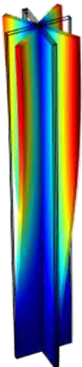
Pure torsional buckling of an X-beam. \sigma_{cr} = 60.2 MPa. (End-load is thrust force and clamped on the other end.)
