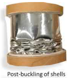
Post-buckling of shells
