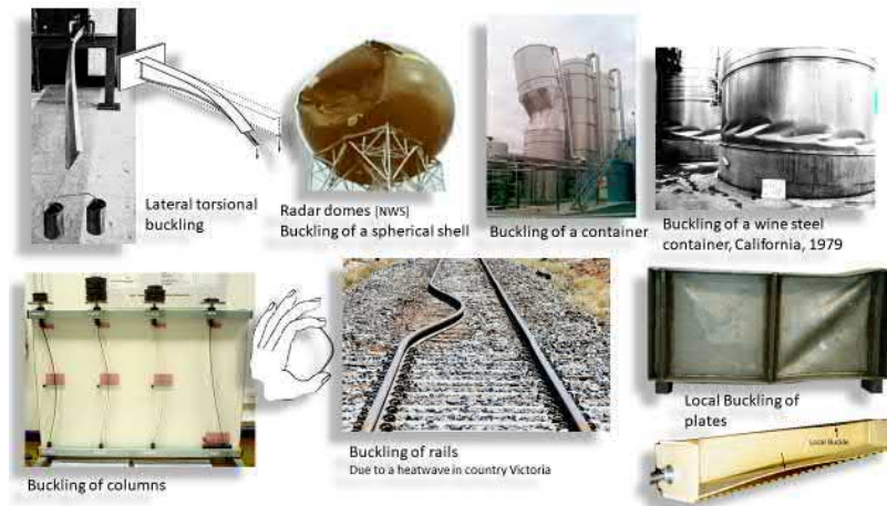
Figure 1.4: Examples of various types of loss of stability in simple structures. From left to right: lateral-torsional buckling, buckling of spherical and cylindrical shells, buckling of slender columns, buckling of a rail-road rail bonded to a support and plate buckling represented by shear buckling of the flanges and compressive buckling of web.
