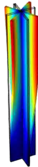
Pure torsional buckling of an X-beam. \sigma_{cr} = 60.2 MPa. (End-load is thrust force and clamped on the other end.)
