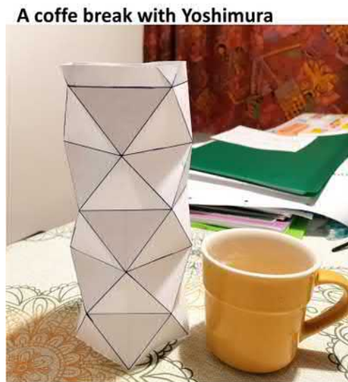
Figure 1.247: A small paper model of Yoshimura buckling patters. Note that the faces of the small triangle are flat. Bending occurs only along the edges of the triangle. This mode, minimises the strain energy, for sure. Just compared to the unstable mode of the chess-board pattern.
