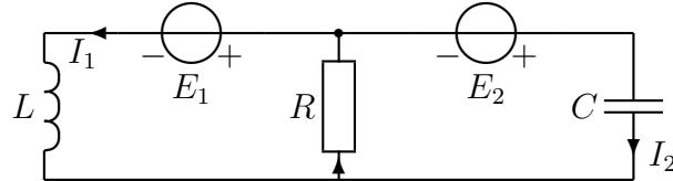
$$-\text{j}\omega L I_1 - E_1 - R(I_1 + I_2) = 0 \Rightarrow I_1 = -\frac{E_1 + RI_2}{R + \text{j}\omega L} \quad (6)$$
