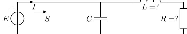
$$S = EI^* = E \left( \frac{E}{\frac{1}{\text{j}\omega C}} + \frac{E}{Z_{LR}} \right)^* = E(E\text{j}\omega C + EY_{LR})^* \quad (12)$$
