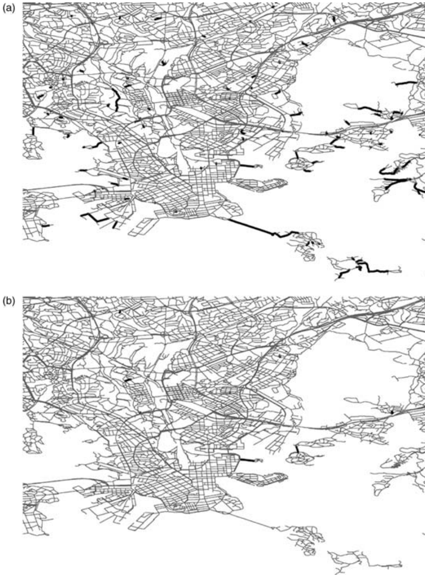
Figure 9 Cut vertices in the centre of Helsinki for (a) k=1 and (b) k=5 . Road segments corresponding to cut vertices are shown as wide black lines, those that correspond to qualified vertices as light grey lines and edges that do not belong to biconnected components of the minimum size in dark grey
