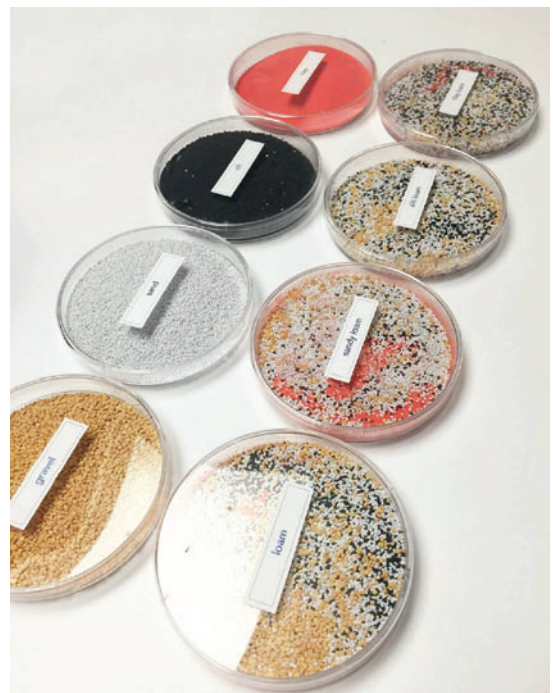
FIGURE 4.3.9 Engineered soil samples. The following “sediments” were used in the live-modeling of the fluvial morphology of riverine systems, which are based upon the weights of the corresponding compositions of varying soils that were analyzed: gravel, sand, silt, clay, loam, sandy loam, silt loam, and clay loam
