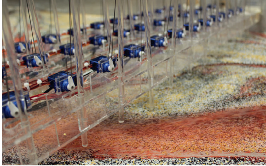
FIGURE 4.3.6 Attuner, a real-time responsive model that monitors and modifies the alluvial morphology of sedimentation based on the fluvial flux of water, resulting in land accretion. It constantly learns from its environment and context through a feedback loop Model: Leif Estrada; photograph: Robert Tangstrom, https://vimeo.com/166623512
