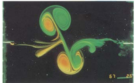
Plate 1 When two dipolar vortices collide, the structures maintain their integrity. The mushroom-like heads exchange vortices and set off in new directions. Here they have been coloured with dyes so that they are identifiable. (Photos: Gertjan van Heijst and Jan-Bert Flór, University of Utrecht.)
