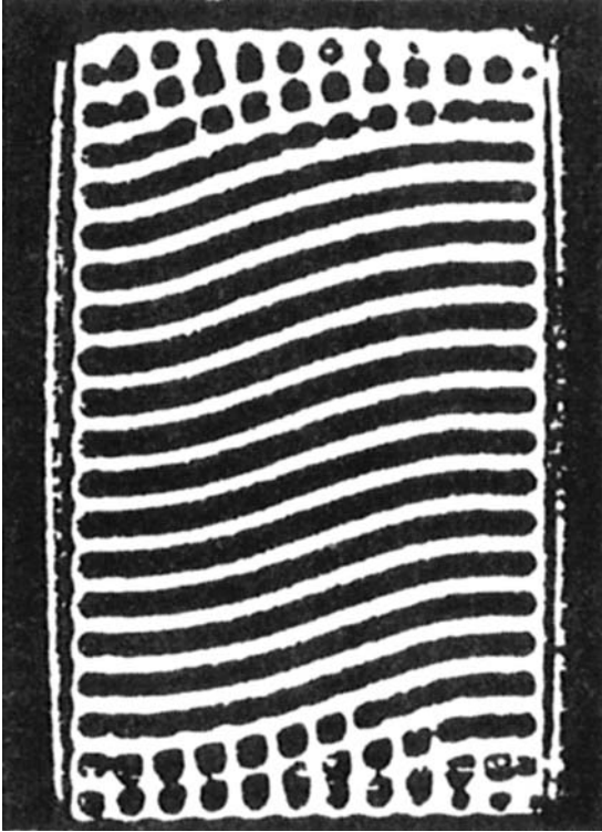
Fig. 3.4: Convection cells in a rectangular vessel. Parallel roll cells are commonly distorted by the vessel's edges. Here the rolls have a slight wavy undulation, and at the ends of the vessel they break up into square cells. (From Cross and Hohenberg, 1993, after LeGal, 1986.)
