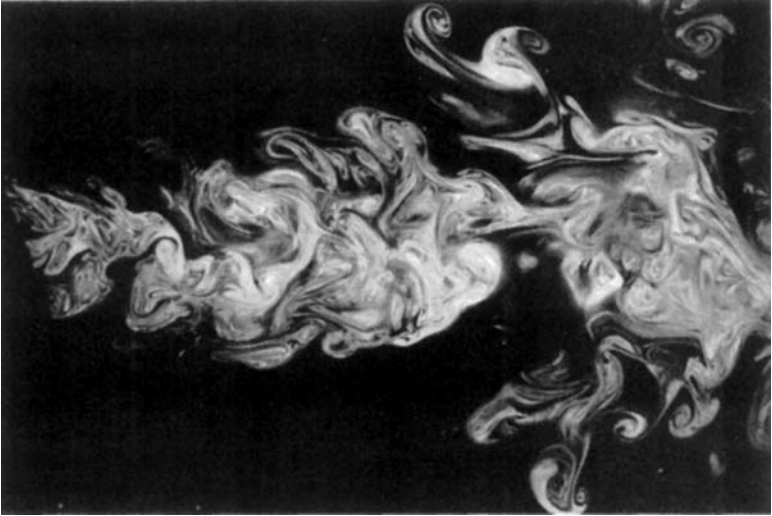
Fig. 6.1: In turbulent flow, the motion of the fluid is chaotic, and yet some coherent structures such as vortices survive. (Photo: Katepalli Sreenivasan, Yale University.)
