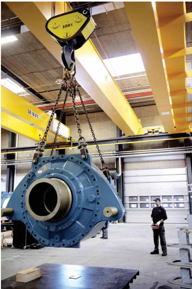
Figure 2. Operating an EOT crane in a factory.
