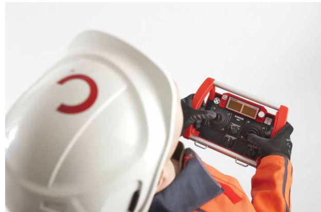
Figure 3. The crane controller.
