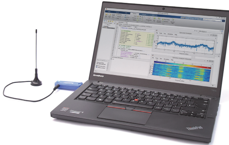
Figure A.1: The NooElec NESDR Mini 2 with antenna connected, plugged into the USB port of a laptop
