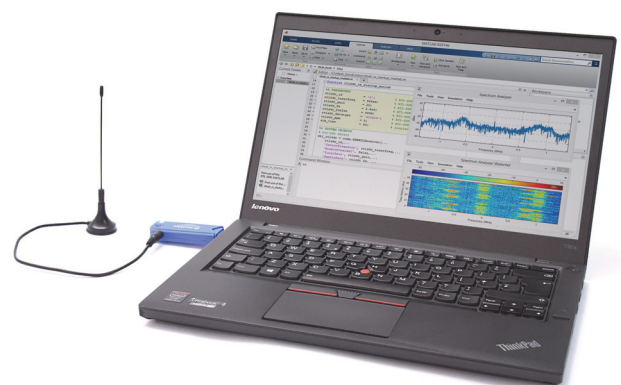
Figure 1.3: RTL-SDR with an omni-directional antenna connected to a laptop via a USB port. The computer is running MATLAB & Simulink to enable implementation of the DSP and SDR algorithms presented in this book. MathWorks tools can be used to monitor the signal in the frequency and time domains as it is demodulated [59]
