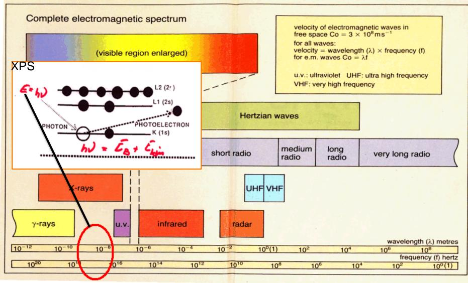
\* In photoelectric effect, X-ray waves 1...100 nm  $\cong$  10..1500 eV, which matches binding energy of core orbitals.
