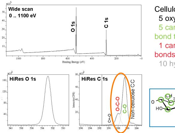
Cellulose molecule: 5 oxygen atoms 5 carbon atoms with one bond to oxygen neighbor 1 carbon atom with two bonds to oxygen neighbors 10 hydrogens (not seen XPS)
