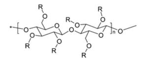
Cellulose R=H Trimethylsilyl cellulose R=Si(CH<sub>3</sub>)<sub>3</sub> Cellulose triacetate R=COCH<sub>3</sub>
