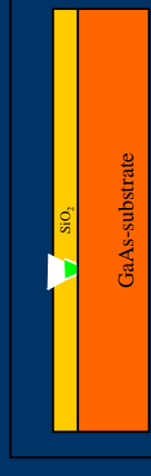
Fig. 6 The onset of QD growth inside the dimple
