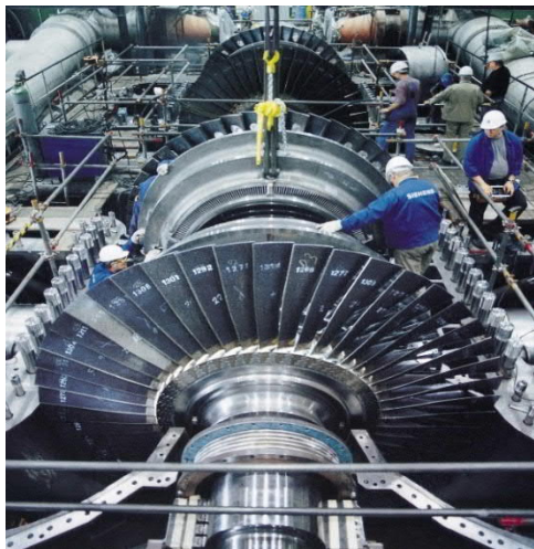
Figure 8.3 Steam turbine plant (Image credit : https://en.wikipedia.org )
