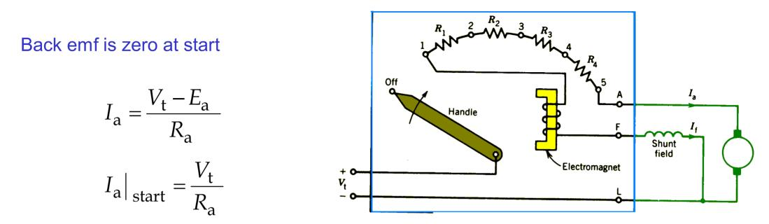
• Variable external resistance is used to reduce the starting current
