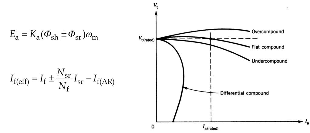
differential compound machine has almost constant current
