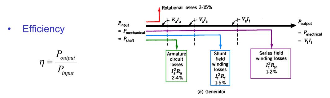
• Core losses are included in the rotational losses
