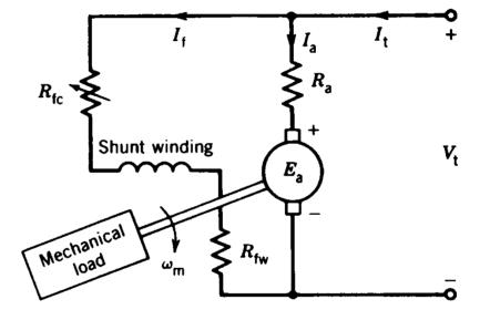
• Armature current and speed depend on the mechanical load
