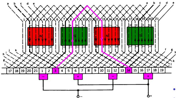
p/2 coil connected in series between two adjacent commutator bars
