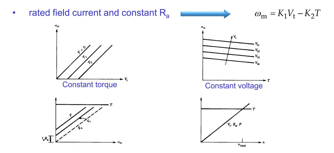
• In actual applications  $I_a$  is kept constant (needs closed-loop operation)  $T = K_a \Phi I_a$   $\longrightarrow$  Constant torque
