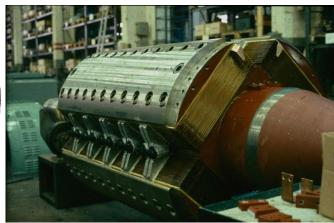
Salient pole machine Non-uniform air gap
