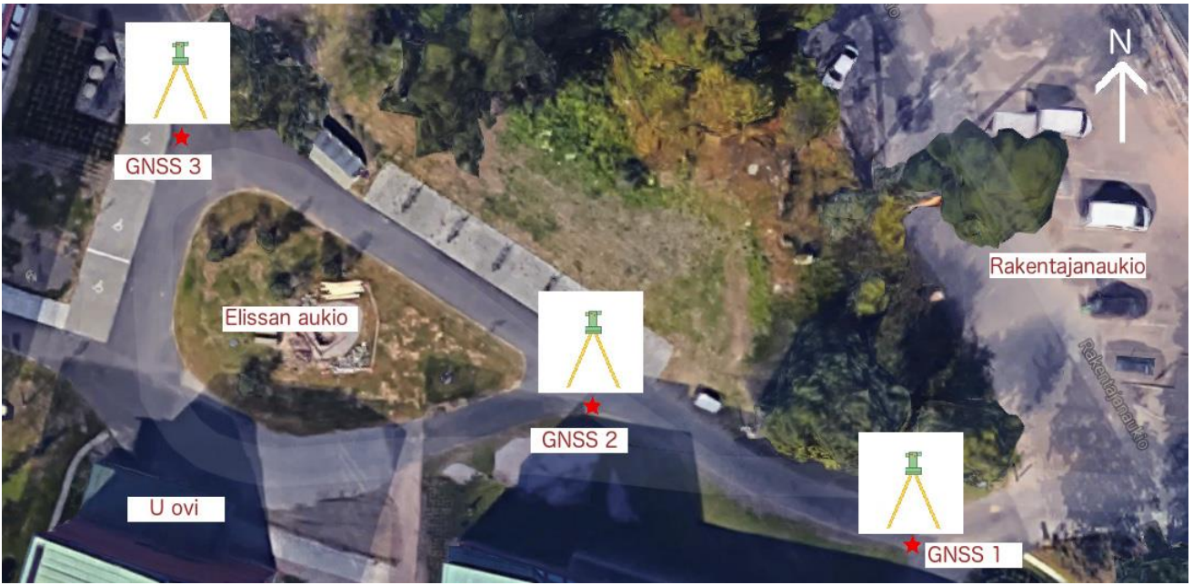
Figure 4: All tacheometer stations have been determined, the mapping can start.
