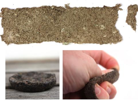
Figure 6. Three selected samples to be used in the product concept creation: CapPurcino (below left), Cofflexi (below right), and Café Maché (above).
