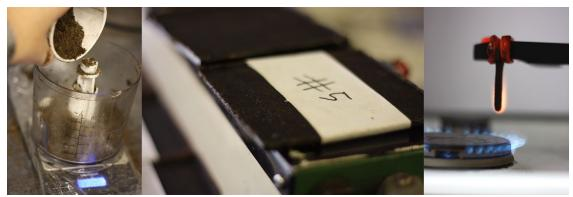
Figure 2. Tinkering with the material: varying the amount of coffee grounds in different samples to be subjected to mechanical tests (left and middle); fire resistance test (right).
