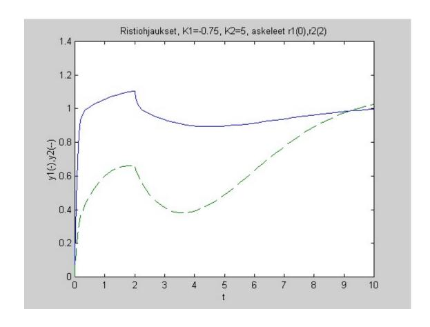
Analysis will later show that the difficulties are because the system has a RHP-zero (zero in the right half plane).
