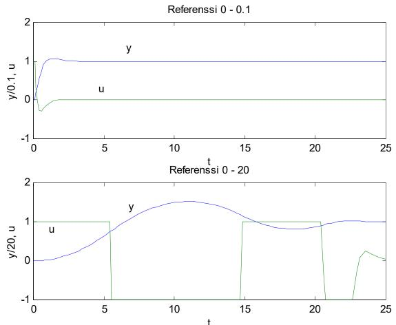
The output deteriorates clearly because of the control signal limitation.
