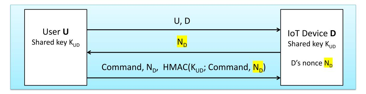
U → D: U, D D → U: N<sub>D</sub> U → D: Command, N<sub>D</sub>, HMAC(K<sub>UD</sub>; Command, N<sub>D</sub>)
