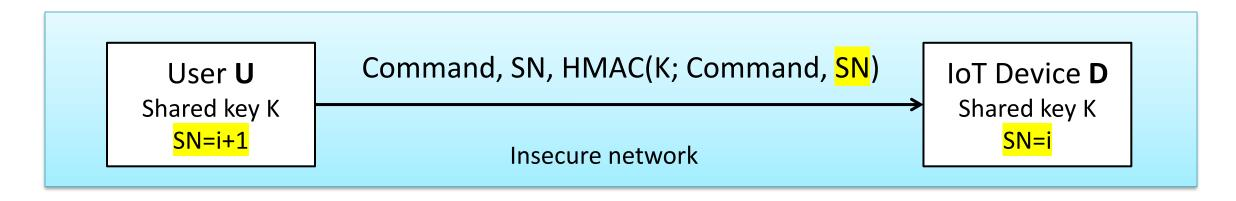
$U \rightarrow D$ : Command, SN, HMAC(K; Command, SN)
