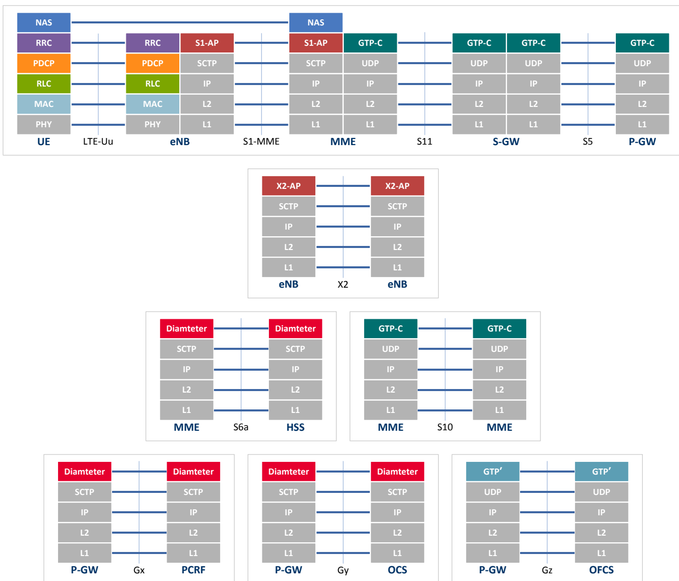
Figure 3. LTE control plane protocol stacks
