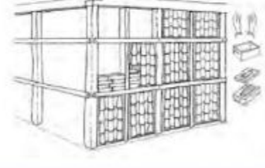
2.7. Half-timber with adobe in fill and tile protection
