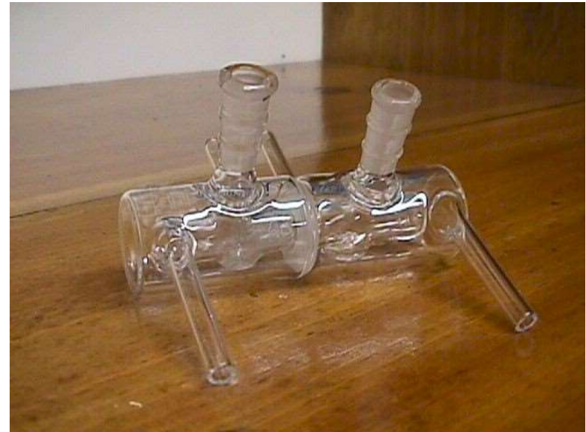
A side-by-side diffusion cell. Total width ca. 9 cm. Chamber volume ca. 3 cm 3 .
