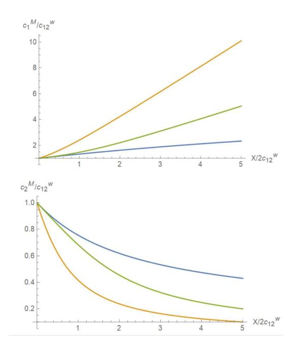
Counter-ion concentrations: 1:1 electrolyte (orange), 2:1 electrolyte (blue), 1:2 electrolyte (green).
