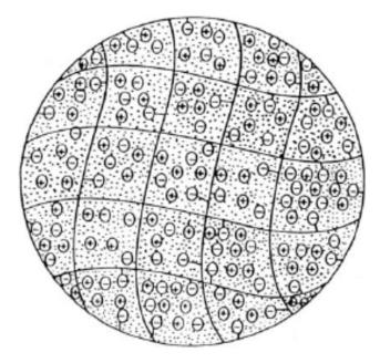
concentration of the fixed groups á dry mass of the matrix because an ion exchanger swells significantly in the solution due to its high ionic strength, causing an osmotic pressure. Ions with a **charge opposite** to the fixed groups are called **counter-ions**, and ions with a **like charge co-ions**. Subscript "1" is used for the counter-ion and "2" for the co-ion.
