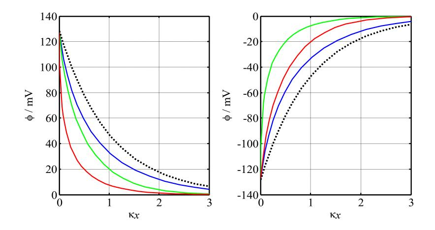
Simulated potential profiles,  $F\phi_0/RT = \pm 5$ : 1:1 electrolyte (blue), 2:1 electrolyte (green), 1:2 electrolyte (red). Black dotted line depicts the linearized equation (10.14). When  $\phi_0 > 0$ , 2:2 electrolyte curve almost coincides with the 1:2 electrolyte curve (red), and when  $\phi_0 < 0$ , 2:1 electrolyte curve (green). Note how the order of curves is changed with  $\phi_0$ .
