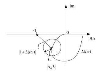
At each point  $L(i\omega)$  a circle with radius  $L\Delta_G$  describes the model uncertainty such that the real curve is ceratinly inside the circle. Assuming that the nominal system is stable (no poles in RHP), the closed loop system is robustly stable exactly when the Nyquist curve does not encircle the critical point (-1,0). That can be expressed as (see figure)
