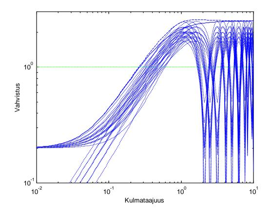
The curve  $l_I(\omega)$  must at each frequency be larger than the dotted curves. It is seen that the value of  $l_I(\omega)$  in small frequencies is 0.2 and 2.5 in large frequencies. For a candidate of  $\Delta_G$  try a first order model, which corresponds to this behaviour
