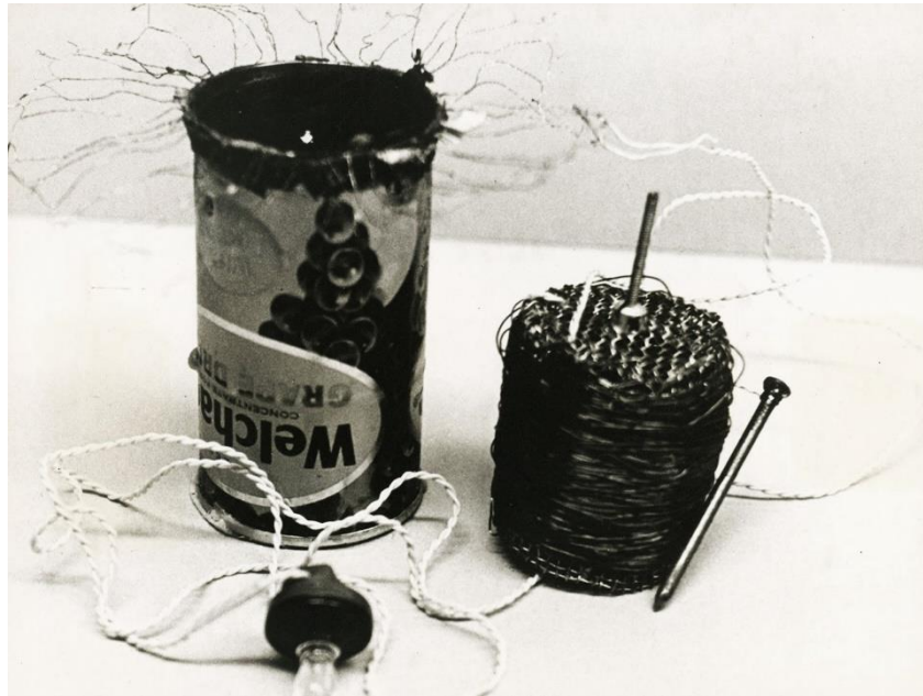
Figure 3: 10 cent tin can radio (Melles et. al. 2011, pp. 225)
