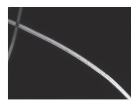
Figure 2 Cotton fiber as seen magnified 10× by a polarized-light microscope.
