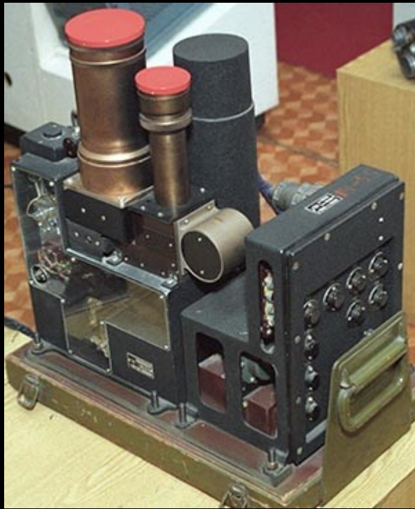
"Yenisey" Phototelevision System, Prototype for AFA-E1
