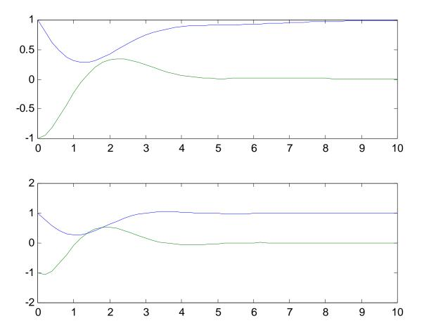
In the lower figure the component  $x_3$  has been given more weight in the criterion.
