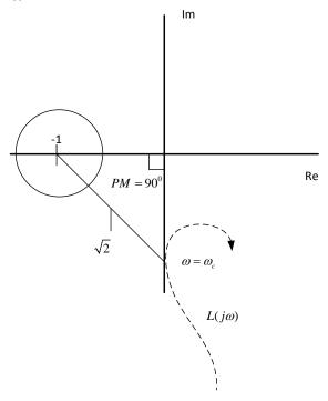
The figure shows the Nyquist diagram of *L* where the phase margin PM = 90 degrees. In the gain crossover frequency then
