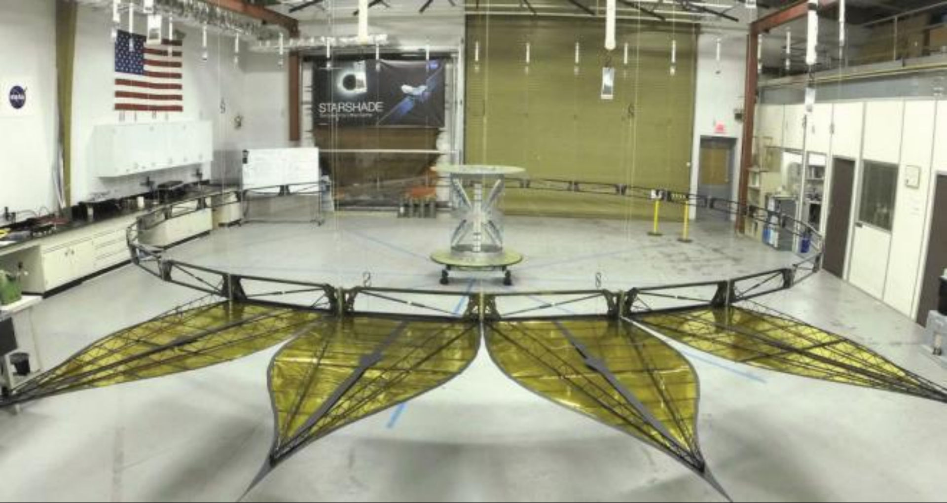
“A 10-m prototype of the starshade’s inner disk is demonstrated at NASA’s Jet Propulsion Laboratory.” (Source)
