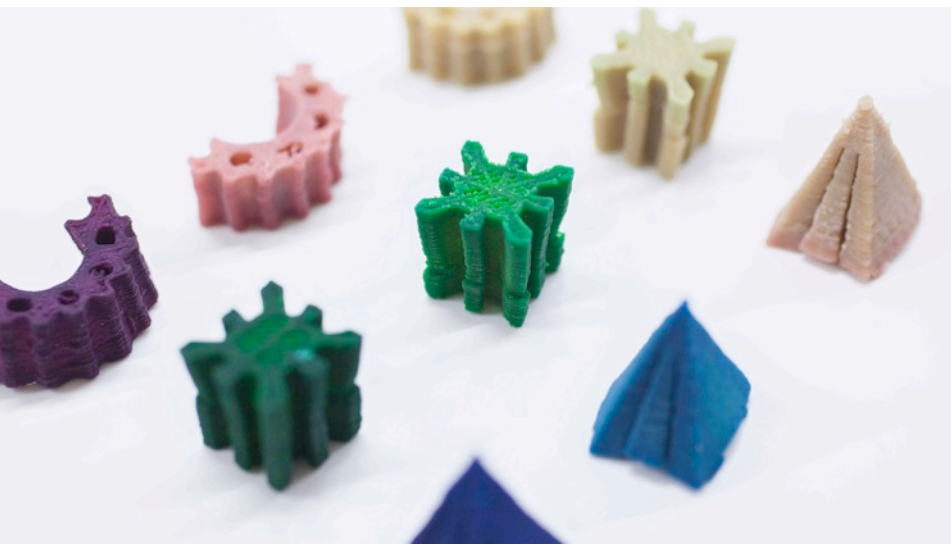
3D printing of cellulosic materials by Anastasia Ivanova and Ville Klar with VTT, DWoC project 2015-2018 Photo Eeva Suorlahti.
