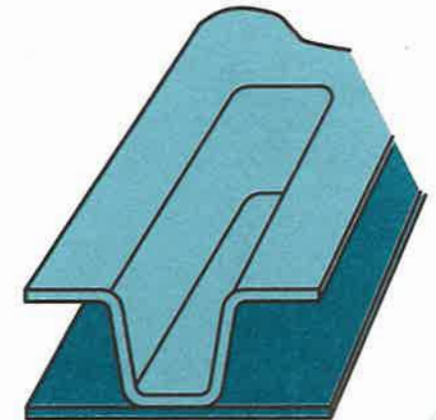
figure 9-45. extrusion blow molding detail: tacked rib (courtesy of Pappago Plastics Inc.)
