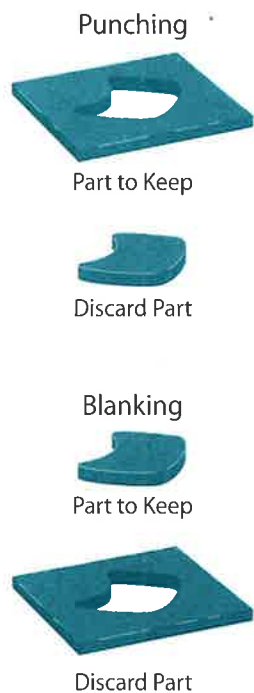
figure 5-3. punch and blank graphic
