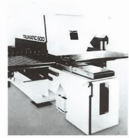
figure 5-8. Trumat 500 punch machine (courtesy Trumpf, Inc.)
