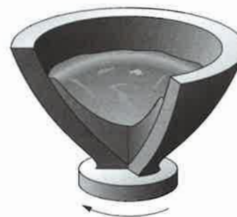
figure 14-23. centrifugal casting of glass
